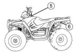
6. **Seat Latch** (6) - The seat latch is under the left edge of the seat. Reach under the left rear fender and pull back on the latch to remove the seat. To replace the seat, set it in place and push down on the seat above the latch. Always make sure the seat is locked in place before riding.
